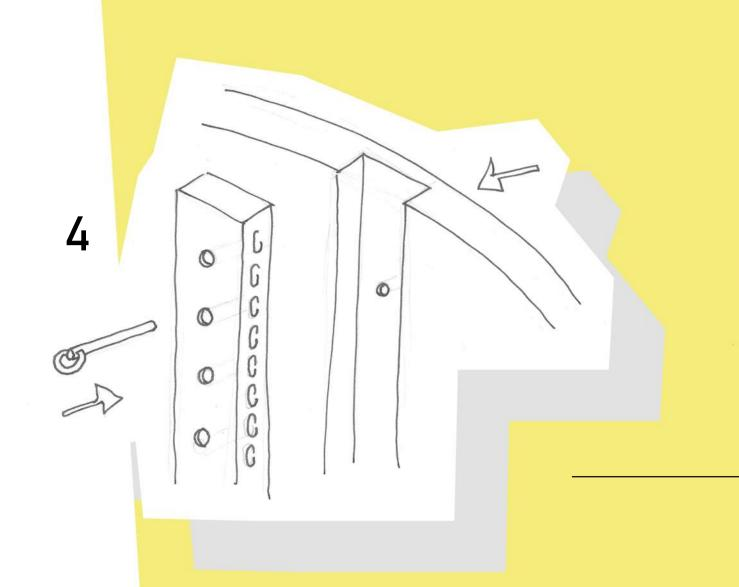
push ly<mark>nch pins</mark> underneath shelf into exis<mark>ting</mark> perforat<mark>ions to</mark> prevent vertical movement\_
